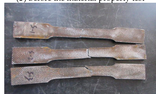
(c) After the material property test
