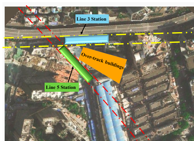
Figure 4. Schematic representation of the over-track buildings and transfer station.
