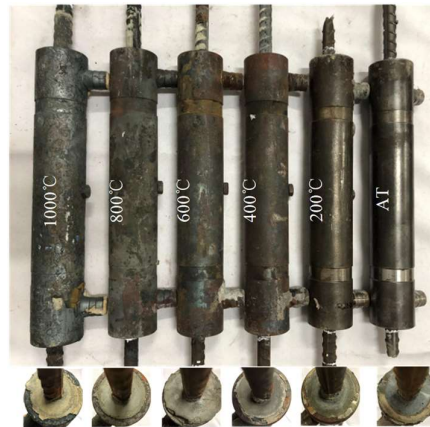
Figure 4. Surface condition of sleeves after heating and water cooling.
