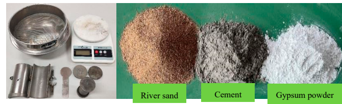
Figure 3. Component materials and tools for specimen fabrication.
