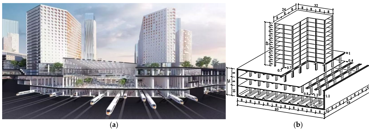
Figure 2. Schematic diagram of three-dimensional section of metro station complex structure in TOD mode (unit: m); (a) actual engineering effect drawing; (b) research model.
