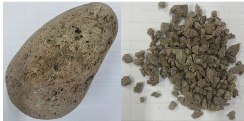
Figure 1. Photographs of a raw pumice stone before and after crushing.
