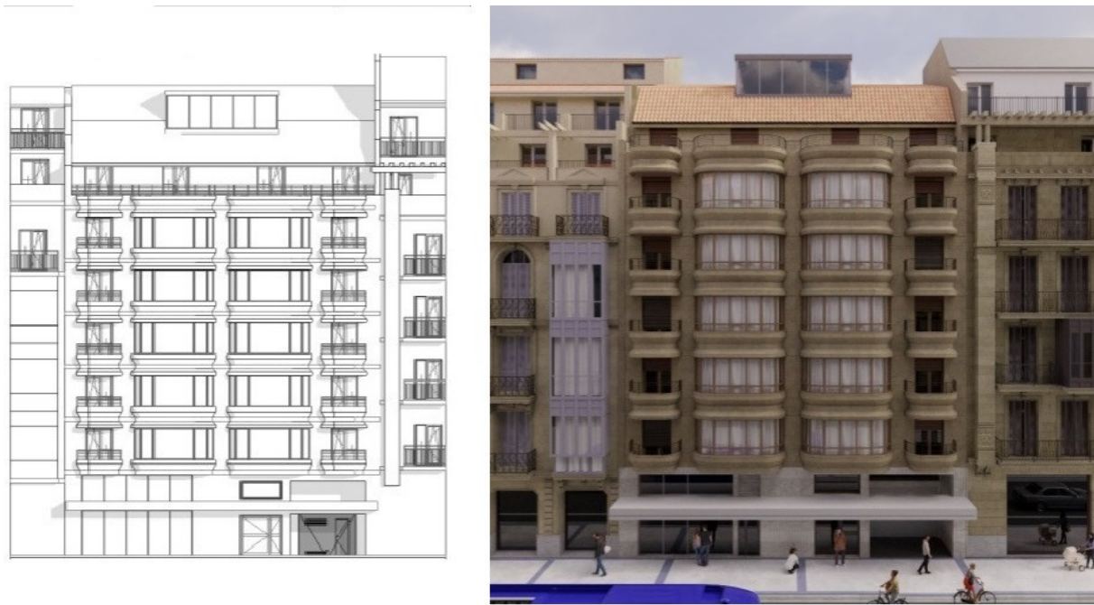
Figure 9. Model of the current state of the facade of the case study in Revit software and rendered image with finishes and textures.
