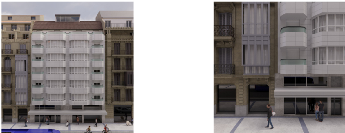
Figure 10. Simulation of a possible intervention of the envelope with the substitution of material and color and simplification of the geometry; cladding detail on the front of the curved balcony and replacement of metal railings with translucent glass.
