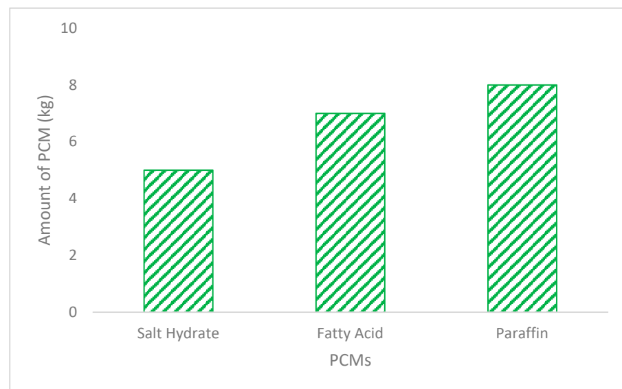
Figure 11. The optimal amount of various PCMs under optical concentration ratio (OCR) of 3.
