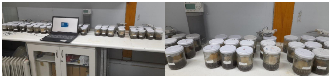
Figure 2. Sealed and conditioned bottles containing the wood samples inoculated for 90 days using the strains taken from Viña del Mar, Nacimiento, Valdivia, and Puerto Varas.
