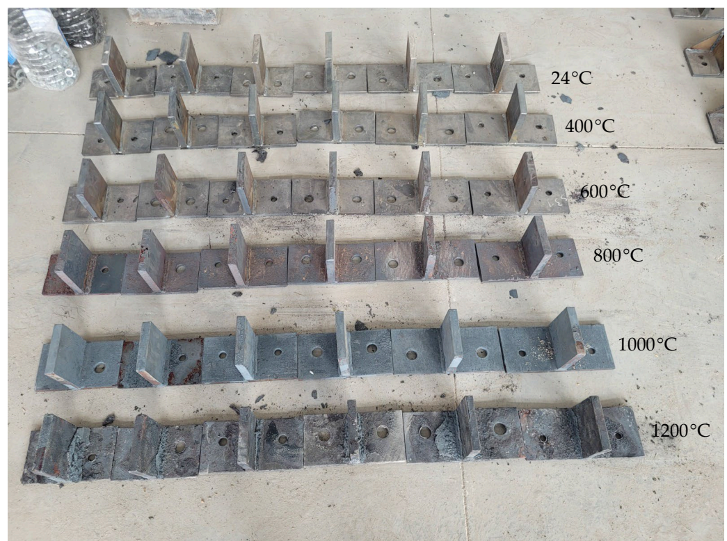
Figure 4. Unheated and heated unstiffened T-stubs.
