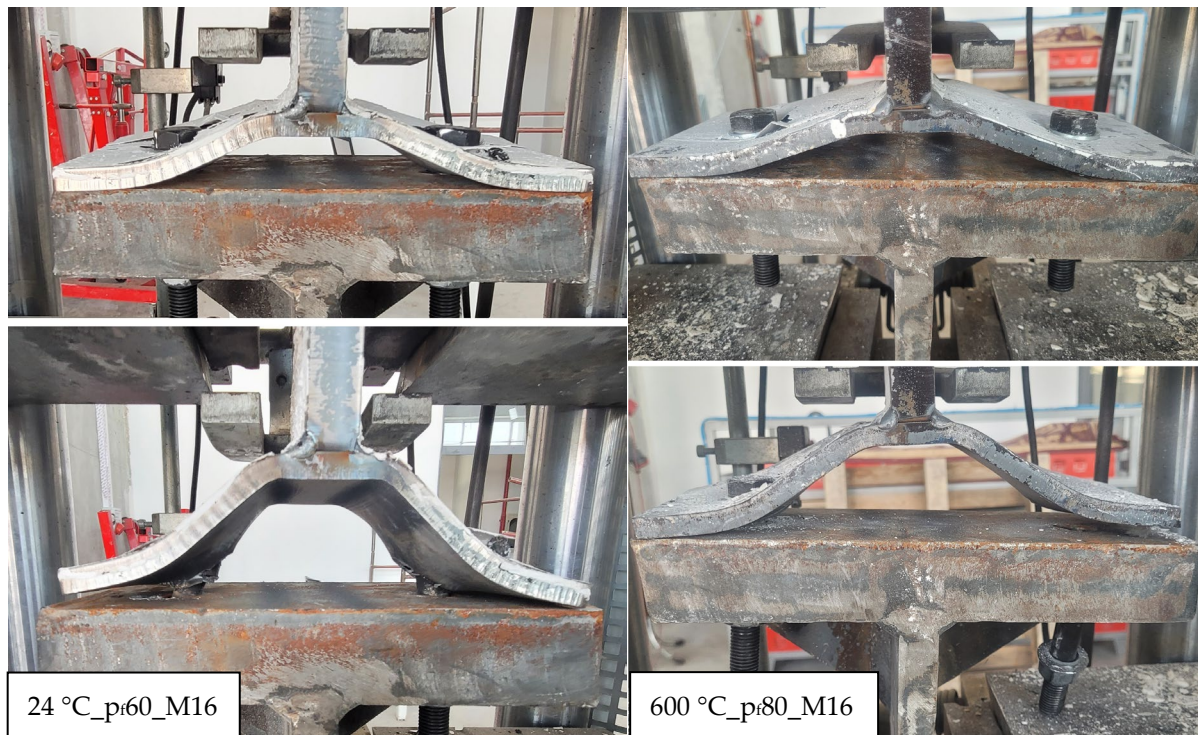
Figure 8. Failure Mode 1 with bolt failure.
