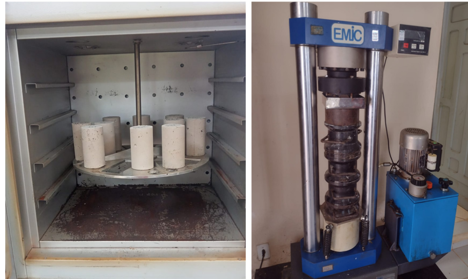
Figure 3. On the left, drying in an oven; on the right, breaking process in a press.
