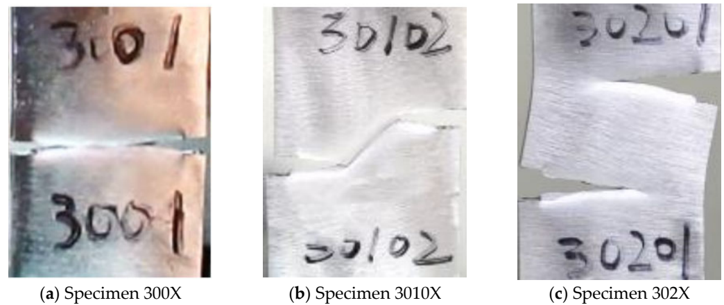
Figure 6. Fracture results of three types of bilateral crack specimens [33].
