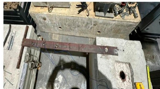
(c) beam with roller support.
