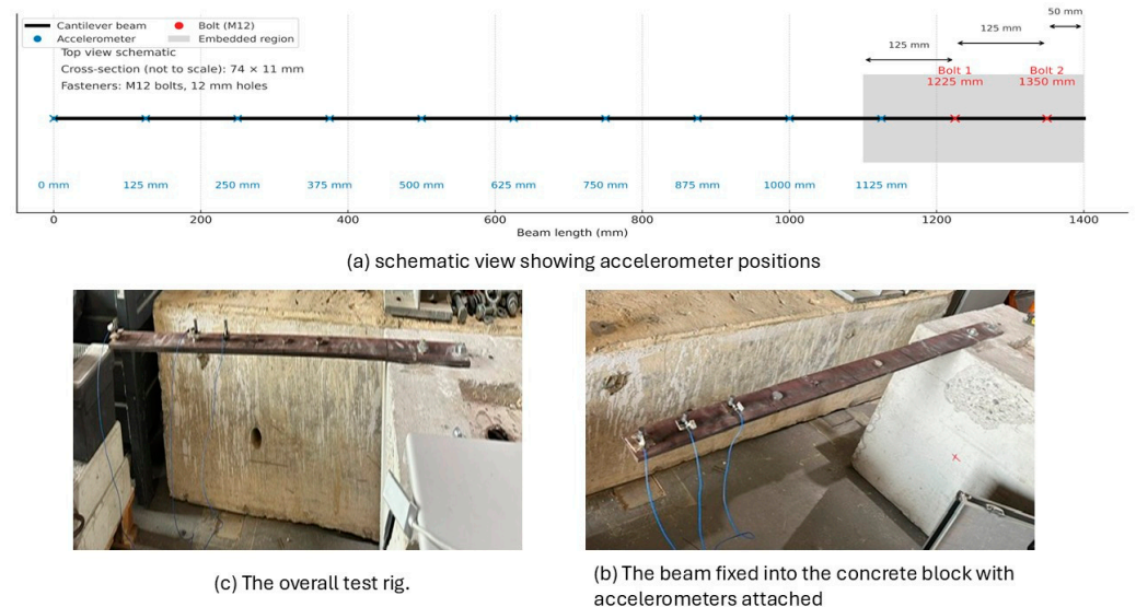
Figure 1. Experimental setup of the steel cantilever beam: (a) schematic view showing accelerometer positions along the 1400 mm beam; (b) photograph of the beam fixed into the concrete block with accelerometers attached; (c) photograph of the overall test rig.
