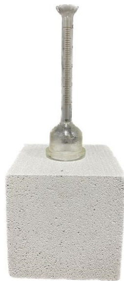
Figure 2. ALC water absorption per unit area test.
