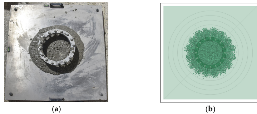
Figure 10. Comparison of J-ring test results and simulation results: (a) test result; (b) simulation result.
