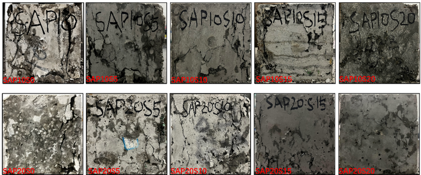
Figure 7. SFRCC compression destruction mode.
