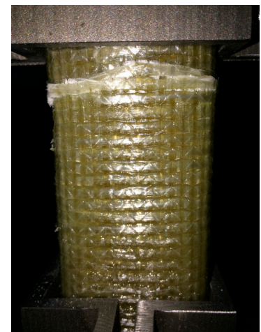
(c) Crushing details at the end of P-sr5-200-3
