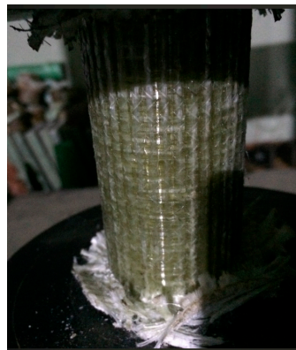
(b) End crushing of R-r5-20-3
