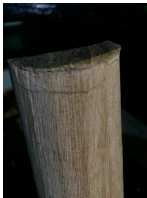
(a) End crushing and wrinkling of R-c-20-3
