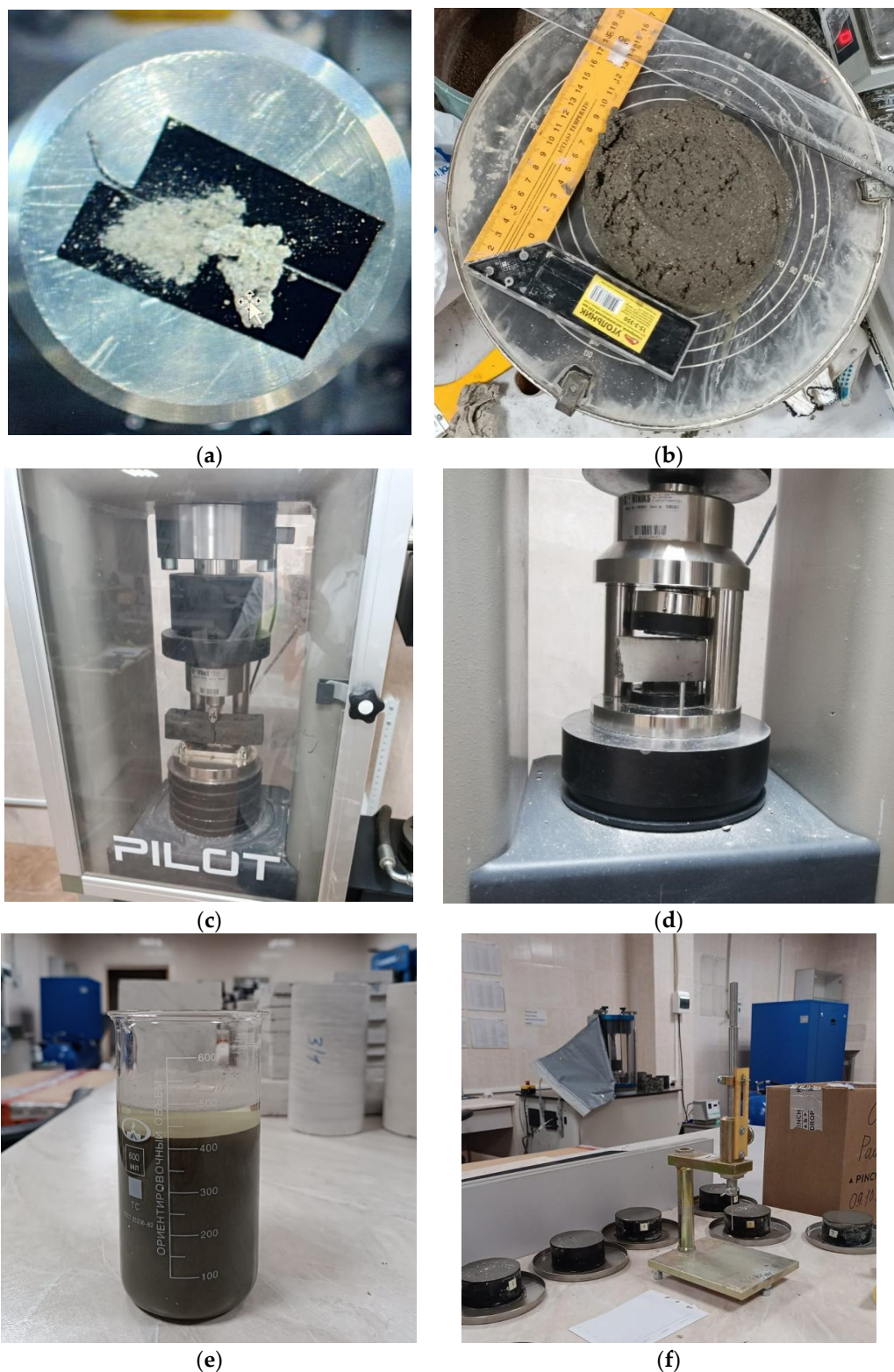
Figure 1. Laboratory testing complex: (a) X-ray fluorescence analysis; (b) the cone spread test; (c) compressive strength; (d) flexural strength; (e) water separation; (f) setting times of cement-sand mixture.
