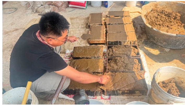
Figure 6. Adobe specimen preparation process.
