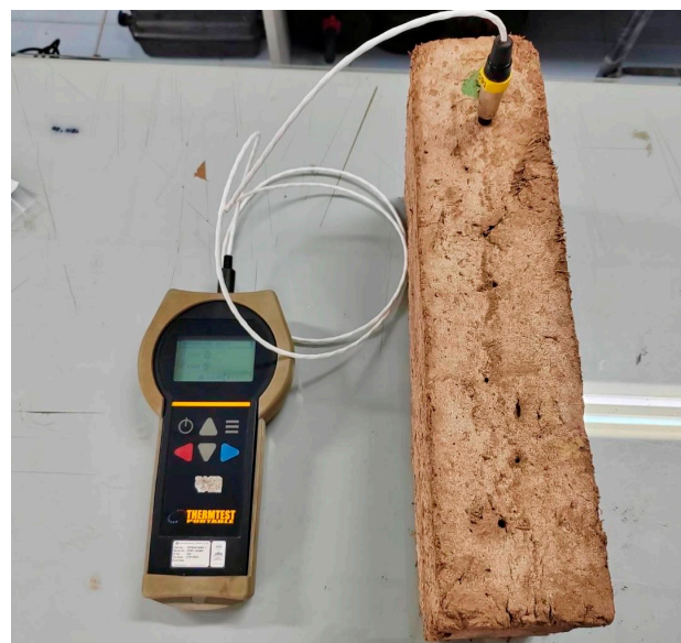
Figure 9. Thermal conductivity measurement using a THERMTEST analyzer with five test locations per full-size adobe brick.
