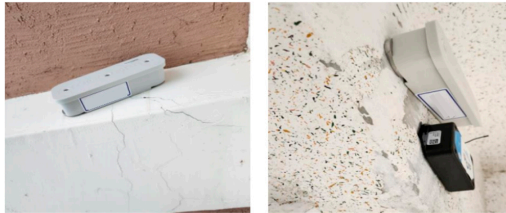
Figure 12. Electronic crack monitoring device used for data acquisition.
