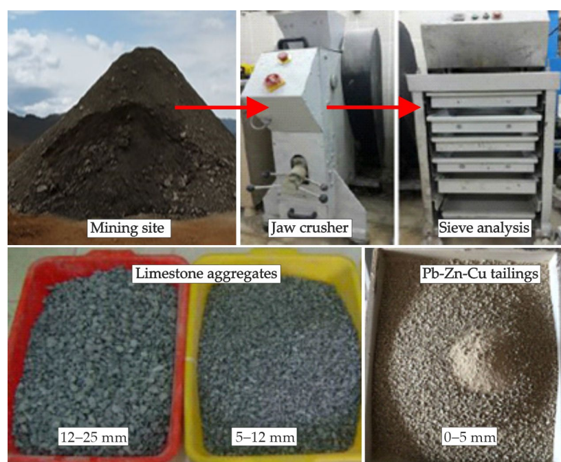
Figure 1. Pb-Zn-Cu tailings and limestone aggregates obtained using jaw crusher and sieve analysis machine.
