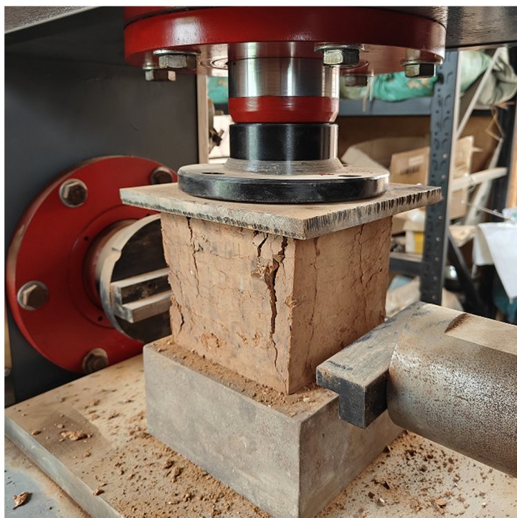
Figure 14. Destructive compressive strength test of RE cube samples.
