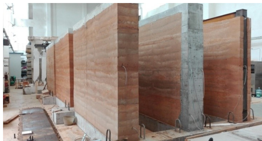
Figure 7. RE wall with top beam and steel cube or concrete structural columns.
