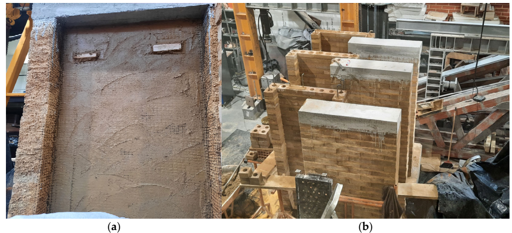
Figure 10. C-panel specimens' construction for in-plane bending shear testing: (a) Plastered C panel; (b) Overview of C panels constructed on the concrete footing.
