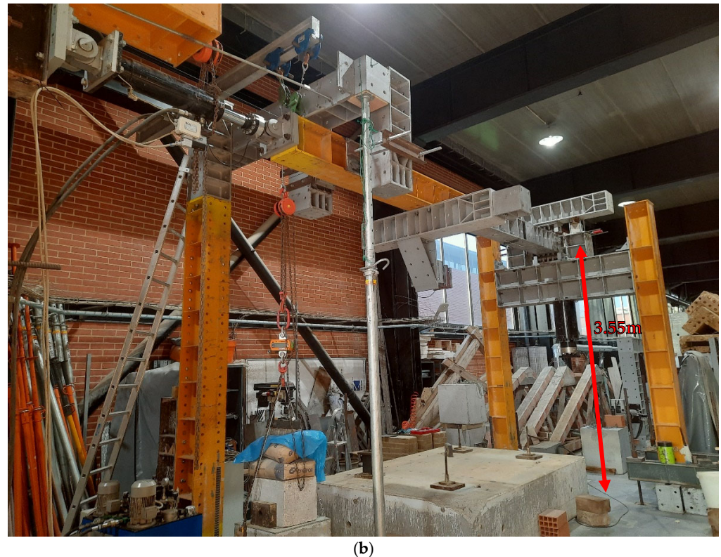
Figure 13. Cyclic bending shear test system for full-scale walls. (a) Illustrating out-of-plane tests. (b) Prepared for in-plane tests. Source: [54].
