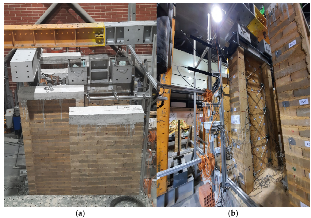
Figure 15. (a) C-panel specimens constructed for in-plane bending shear testing. (b) Instrumented wall for testing.
