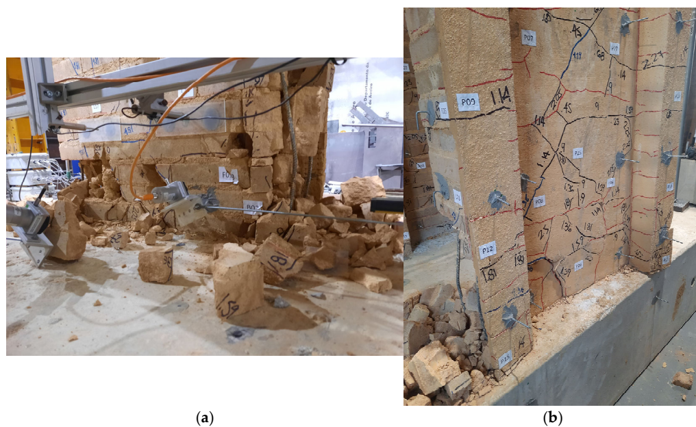
Figure 20. Steel bar buckling and damaged blocks nearby (a,b).
