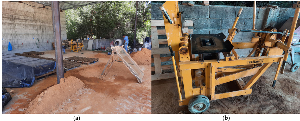
Figure 8. (a) Factory area set up in company Vagoínertes LDA's facilities. (b) Hand mechanical press used to produce bricks.
