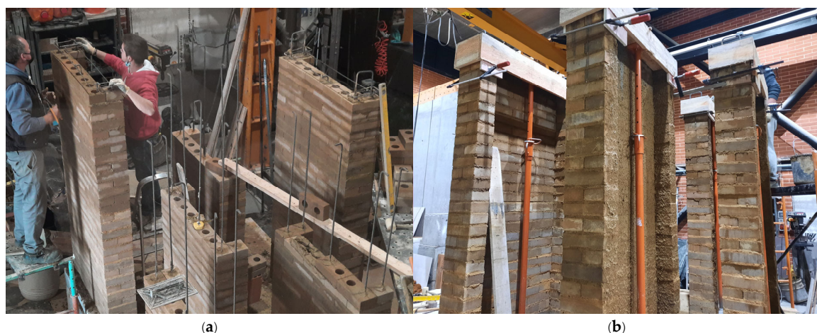
Figure 9. C-panel specimens' construction for out-of-plane bending shear testing: (a) Vertical reinforcements within the blocks' holes; (b) Concrete molding at the panels' top.
