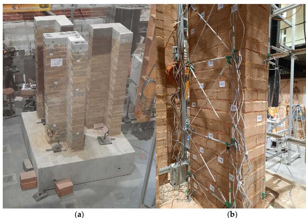
Figure 16. (a) L-panel specimens constructed for in-plane bending shear testing. (b) Instrumented wall for testing.
