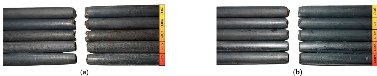
Figure 7. Fracture morphology of high-strength steel wire. (a) With initial stress; (b) without initial stress.
