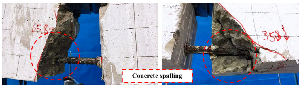
Figure 9. Concrete splitting failure of beam specimen.
