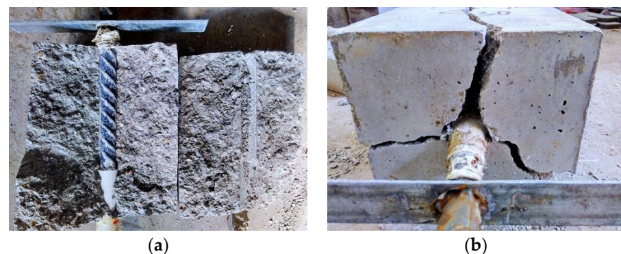
Figure 7. Concrete splitting failure of pull-out specimen: (a) the concrete splits into two pieces; (b) the concrete splits into three pieces.
