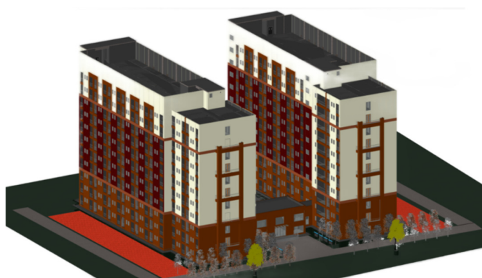
Figure 3. Autodesk Revit 3D Building Model.
