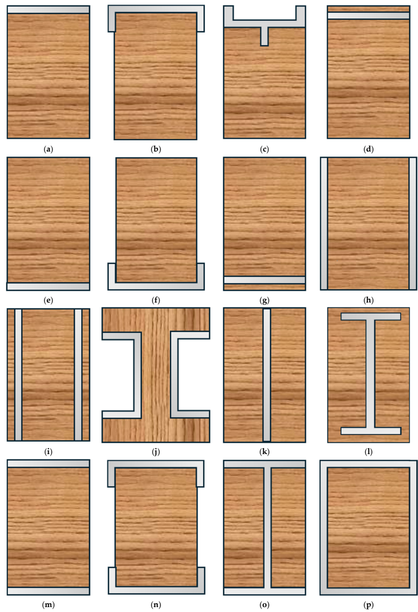
Figure 7. Examples of steel–timber hybrid reinforcement configurations: (a) top flat plate; (b) top U-shaped; (c) top Y-shaped; (d) embedded top; (e) bottom flat plate; (f) bottom U-shaped; (g) embedded bottom; (h) side flat plates; (i) embedded sides; (j) C-shaped sides; (k) embedded middle; (l) embedded I-shape; (m) combined top and bottom flat plates; (n) combined top and bottom U-shaped; (o) combined top, bottom, and embedded; (p) combined top bottom and sides.
