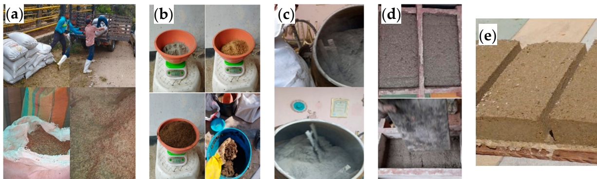
Figure 3. (a) Material processing (grinding and sieving), (b) measuring the ingredients, (c) mixing of dry and wet components, (d) layer compaction and casting, and (e) sun drying of molded bricks.
