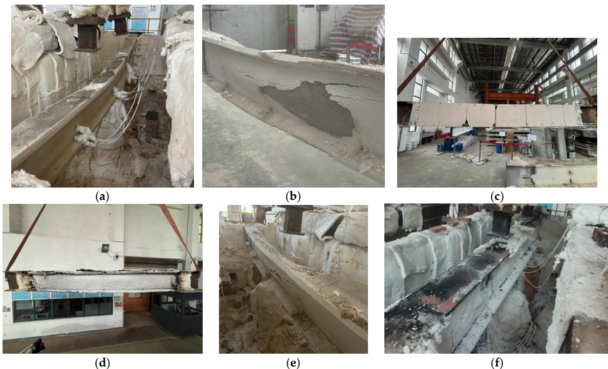
Figure 13. Failure mode of the specimens: (a) D-1; (b) D-2; (c) D-3; (d) D-4; (e) ISO-1; and (f) ISO-2.
