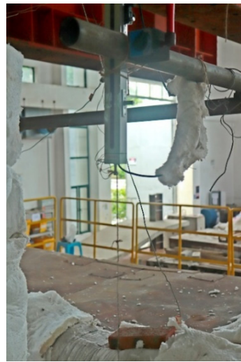
Figure 8. Arrangement of the LVDT.
