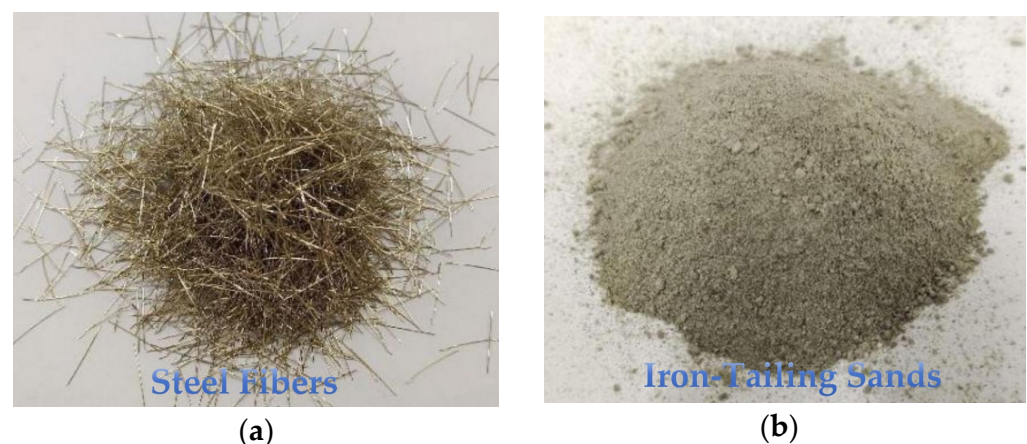
Figure 1. Conductive phase materials: hooked-end steel fibers (a) and iron tailings sand (b).
