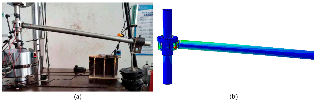
Figure 5. Deformation characteristics of finite element and experimental loading in the final state. (a) Bending test; (b) FE simulation.
