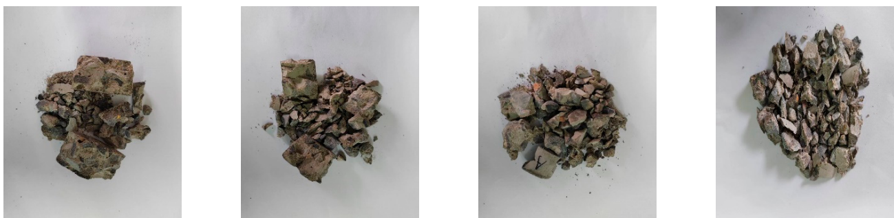
(a) zero freeze–thaw cycles (b) ten freeze–thaw cycles (c) twenty freeze–thaw cycles (d) thirty freeze–thaw cycles
