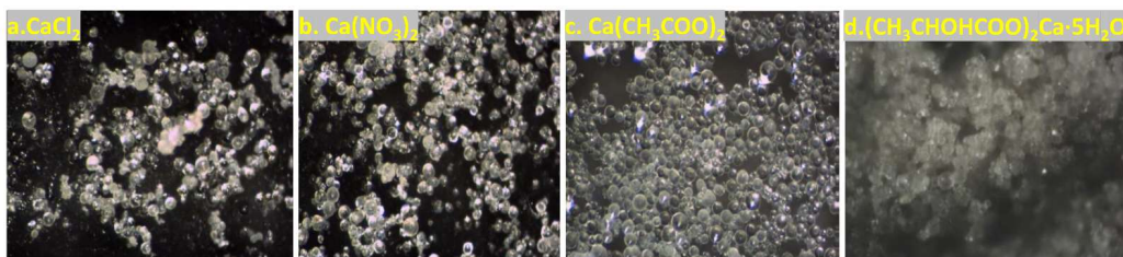
Figure 12. SEM of calcium carbonate minerals corresponding to different calcium sources.
