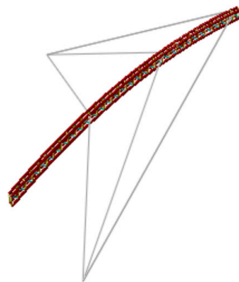
Figure 24. Finite element model of Shenzhen Rainbow Bridge.
