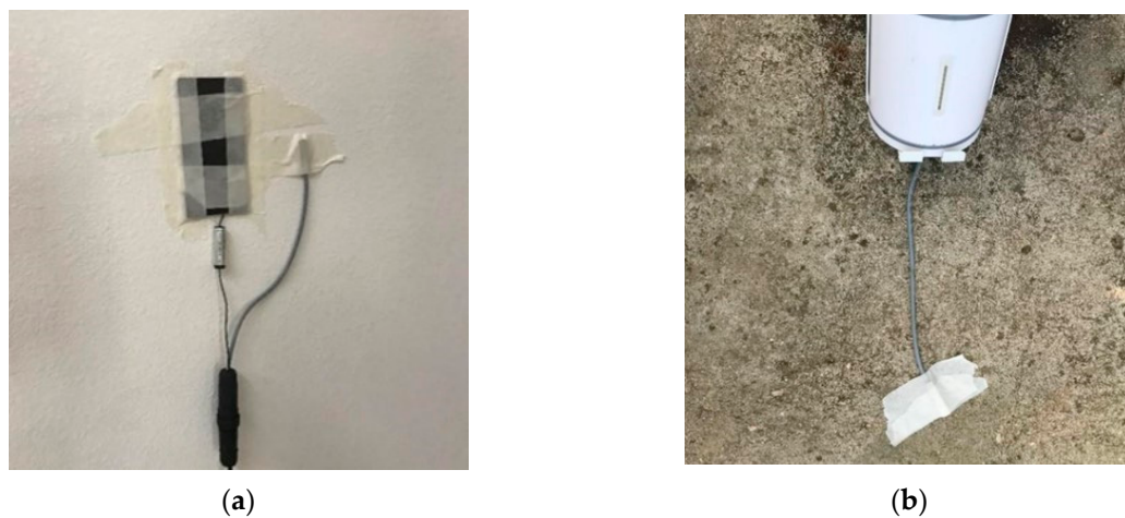
Figure 7. (a) Roof inner surface measurement point; (b) roof outer surface measurement point.
