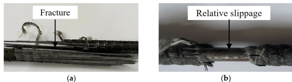
Figure 5. Final failure of GFRP–steel composite bars: (a) RC composite bars; (b) PC composite bars.
