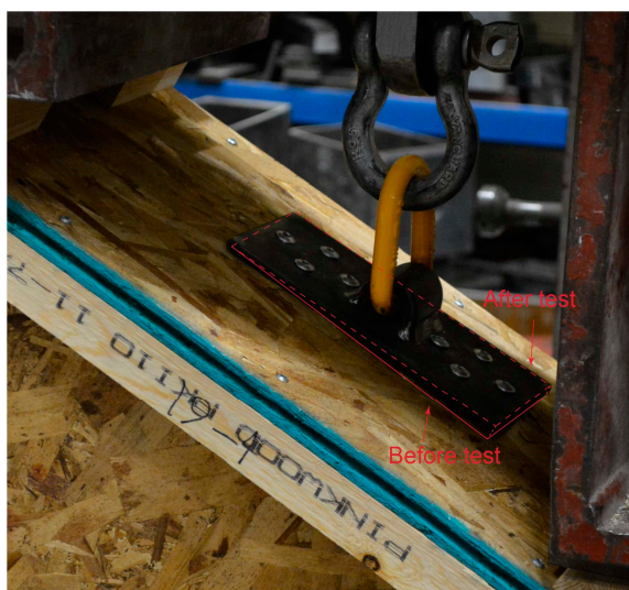
(a) Screw withdrawal and plate lifting
