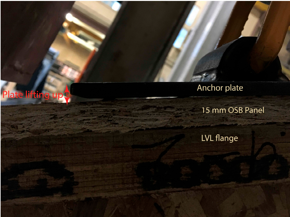
Figure 9. Withdrawal failure of specimen No.9 #2.
