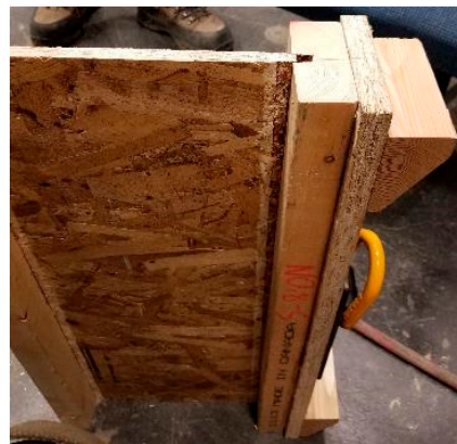
Figure 11. Flange pull-out of No.8 #5.
