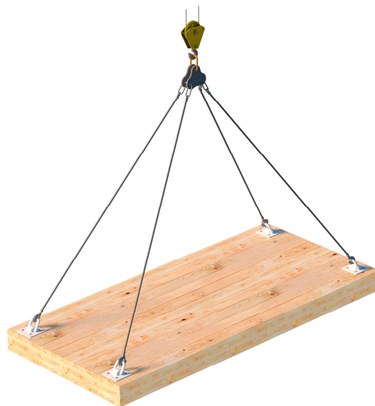
Figure 2. A typical rigging assembly for CLT panels [3].
