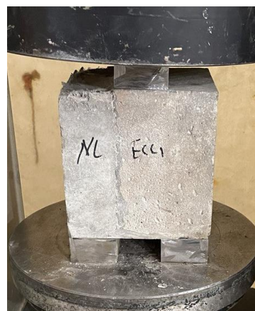
Figure 9. Bi-surface shear test and test setup.
