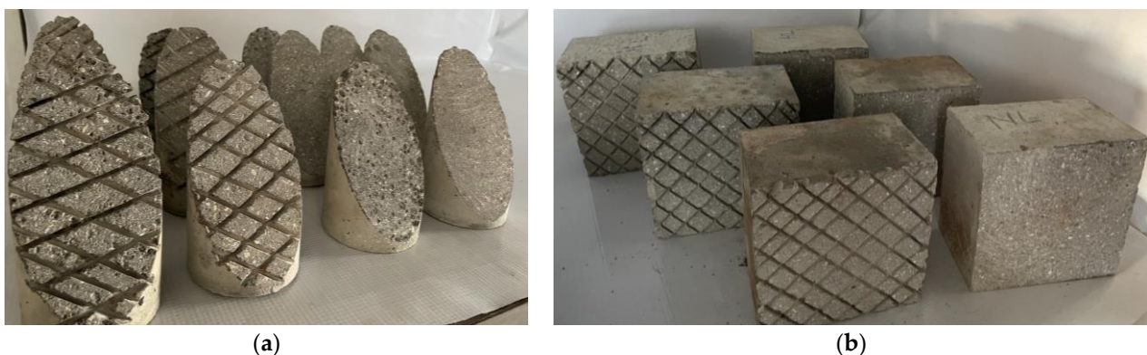
Figure 7. Interface roughness (a) half cylinder grooved and as cast surface and (b) two-thirds of the cube grooved and as cast surface.
