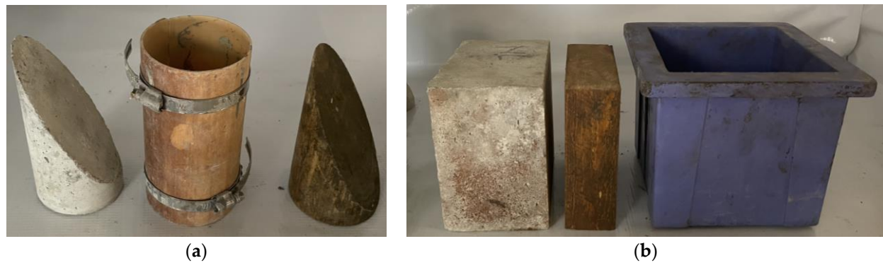
Figure 6. Wood slices for (a) slant shear and (b) bi-surface shear test.
