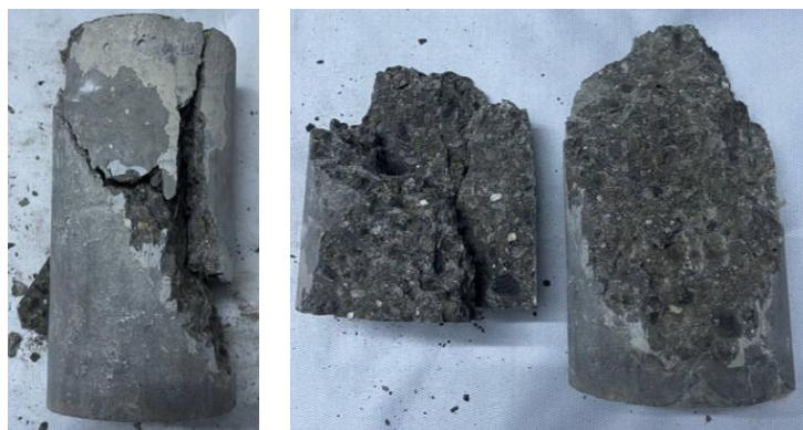
Figure 16. Slant shear typical failure mode D—Complete substrate failure.
