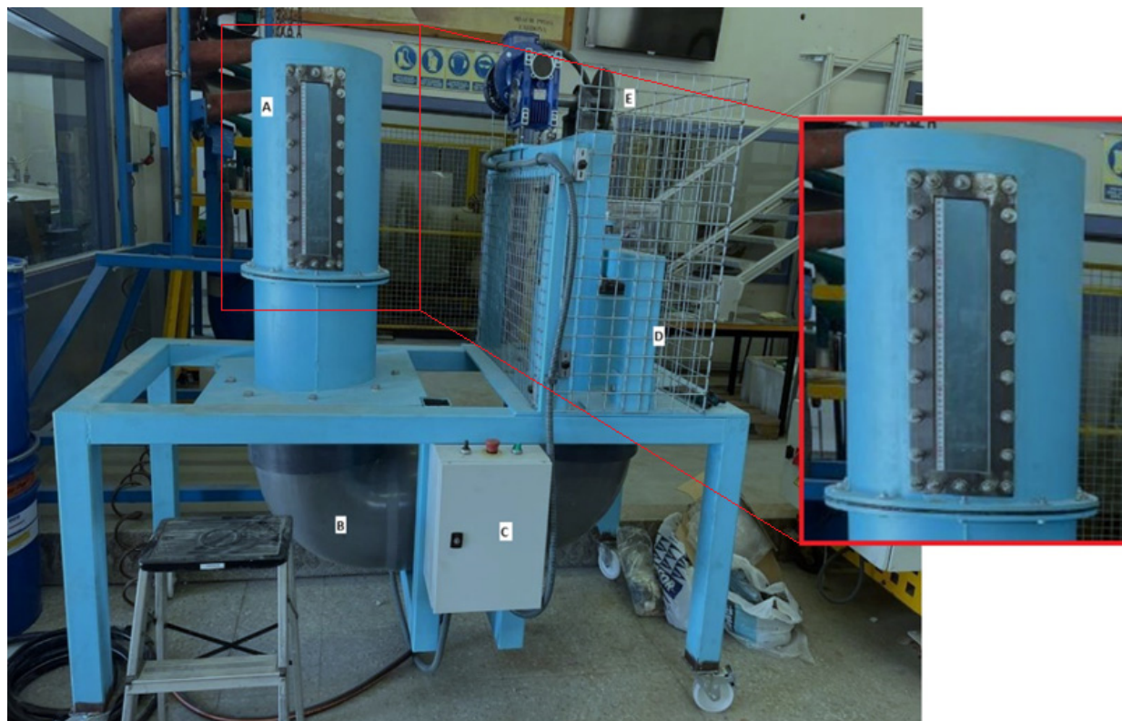
Figure 4. Jig equipment used in the experiments: (A) jig chamber (enlarged), (B) water passage duct, (C) electric panel, (D) pump chamber, (E) motor. Modified from Teixeira et al. [39].
