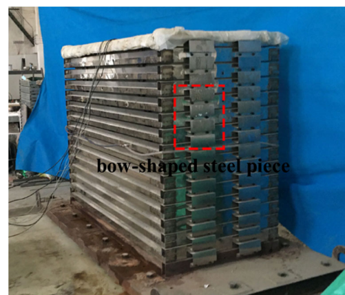
Figure 5. Stratified shearing model box. The red rectangle indicates a bow-shaped steel plate.
