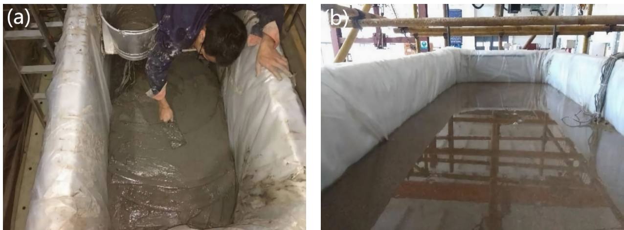
Figure 12. Model making process: (a) reclamation of marine soft soil; (b) the settling of water injection.
