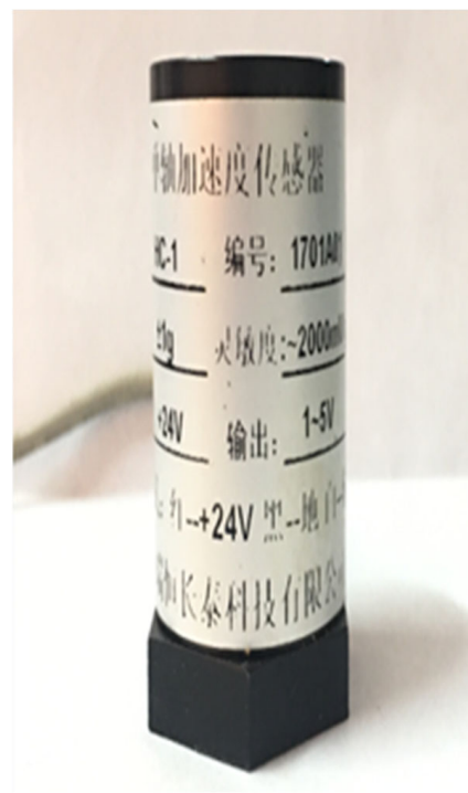
Figure 11. Accelerometer. The inscription above the image denotes a flat-axis accelerometer.
