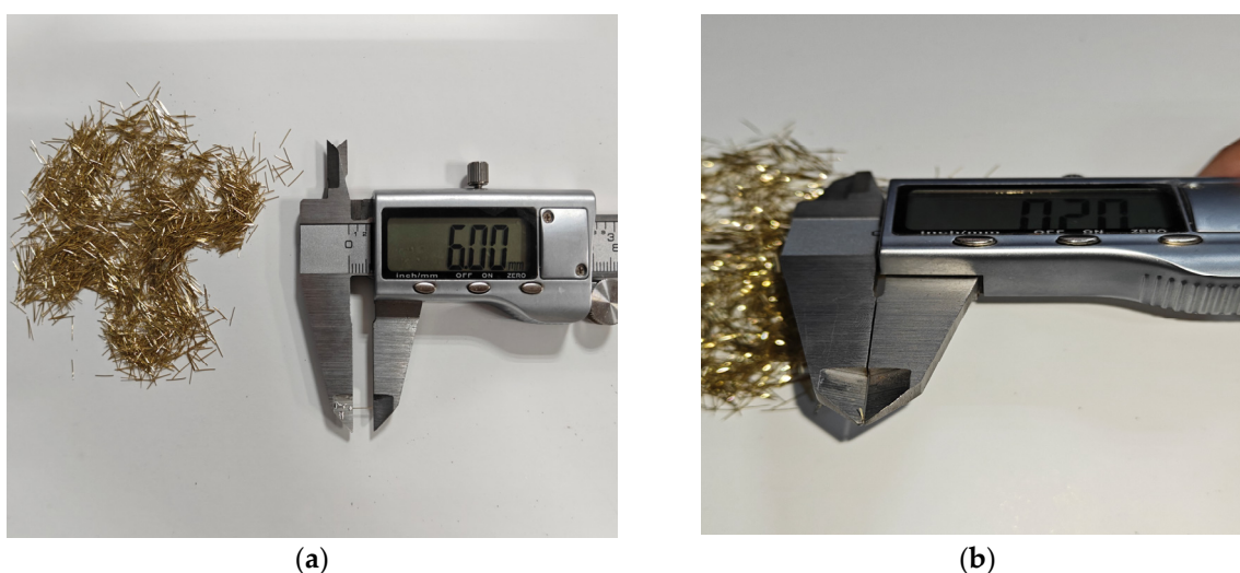
Figure 2. Extra-short extra-fine steel fibers: (a) length; and (b) diameter.
