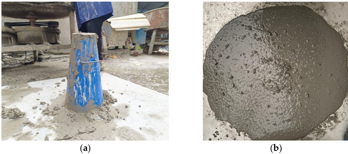
Figure 3. Slump flow test: (a) experimental procedure; and (b) experimental results.
