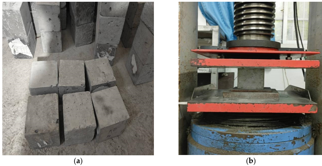
Figure 6. Cube compressive strength test: (a) cubic compressive specimen; and (b) compression test procedure.
