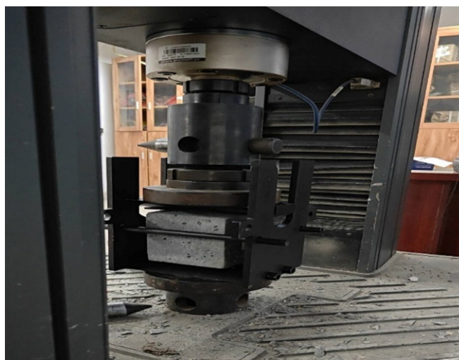
Figure 8. Splitting tensile test.
