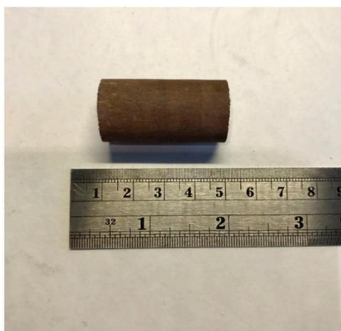
(b) Cylindrical geopolymer sample (length = 40 mm; diameter = 20 mm)
