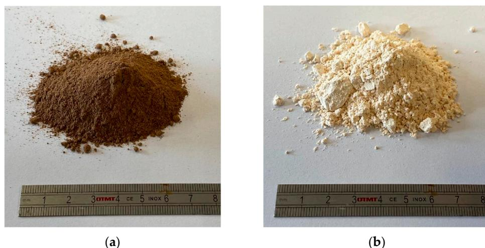
**Figure 1.** Geopolymer precursors: (a) MGS-1 after 6 h of milling with a Bottle Roller and (b) metakaolin after the calcination of kaolinite for 3 h at 650 °C.
