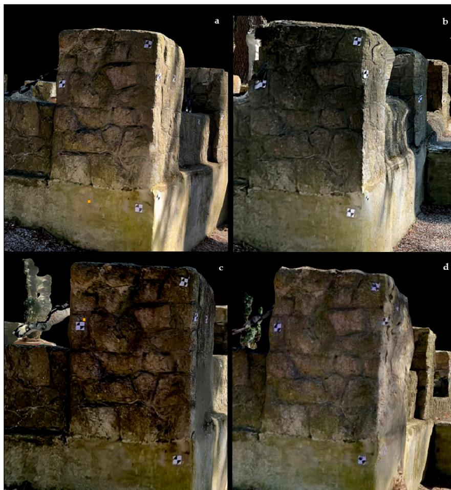
**Figure 12.** Focusing on the edge sharpness and ability to preserve perpendicular parts: (a) Scaniverse, (b) 3DScannerApp, (c) Polycam—LiDAR approach, (d) Polycam—photogrammetry approach.
