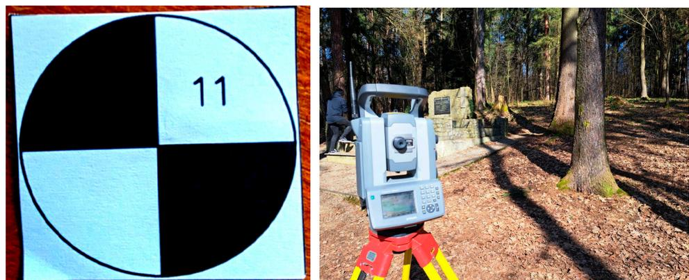
Figure 2. Detailed observation points shape (left), Trimble VX series used for measurement (right).
