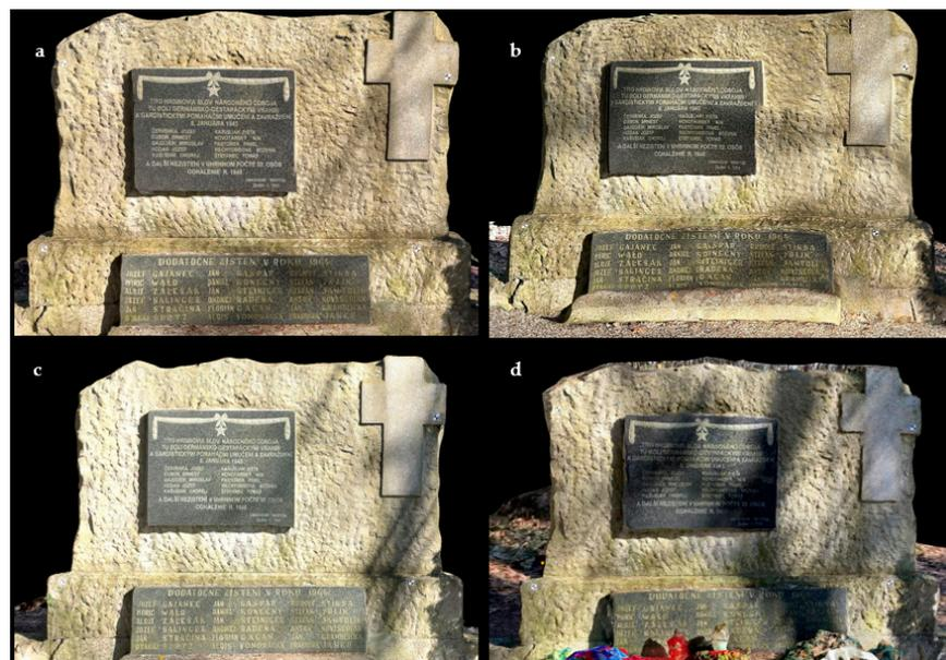
**Figure 10.** Focusing on the detail-capturing ability, shape of the object reconstruction, and distortion occurrence of the resulting 3D models: (a) Scaniverse, (b) 3DScannerApp, (c) Polycam—LiDAR approach, (d) Polycam—photogrammetry approach.
