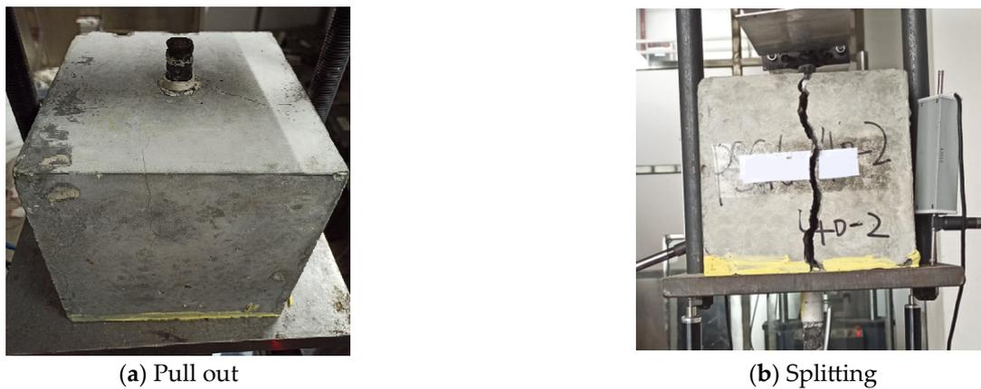
Figure 6. Failure mode.
