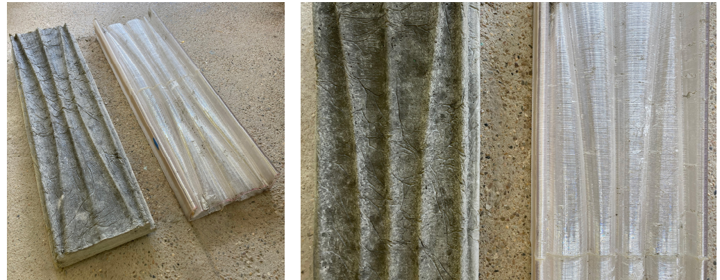
Figure 3. An unreinforced 1.5 m long double-curved concrete component removed from formwork made via PETG robotic extrusion. The creased texture results from a vacuum-bag plastic lining that was used to facilitate demoulding and to protect the PETG.
