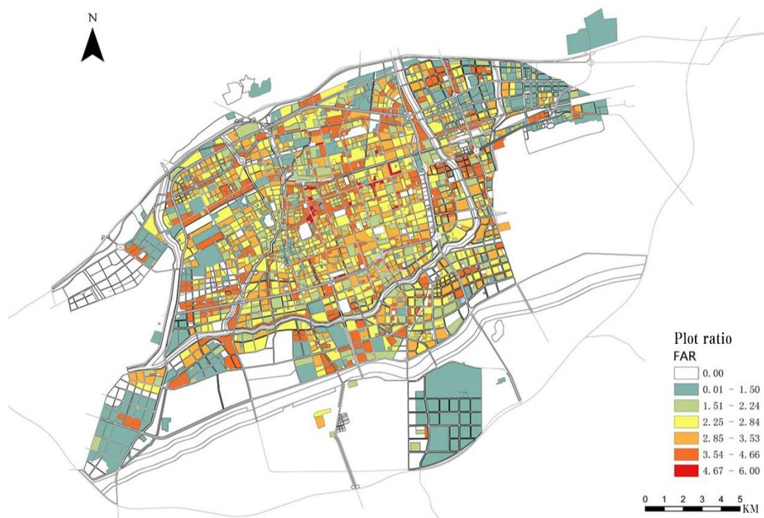
**Figure 3.** Plot ratio simulation results of each block. Source: Drawn by the author. Building density of a certain area.
