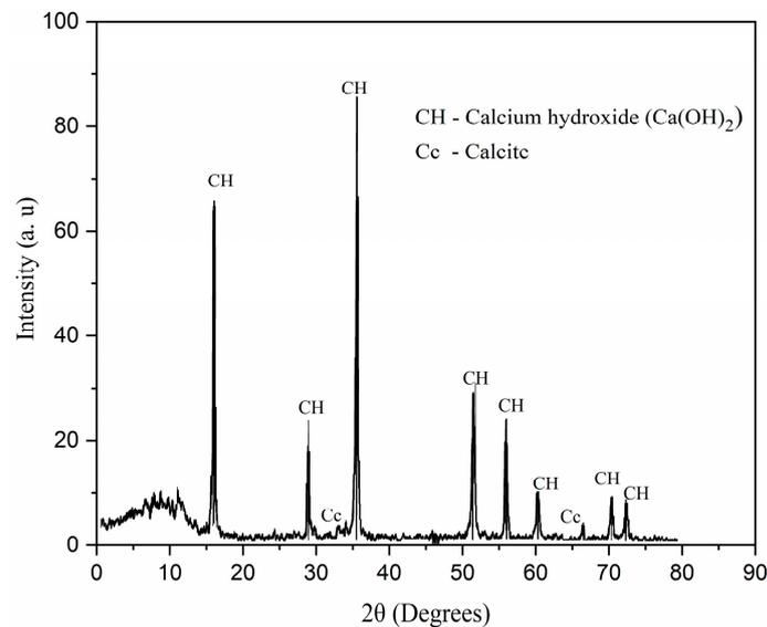
**Figure 1.** XRD of hydrated lime showing the peaks of calcium hydroxide.
