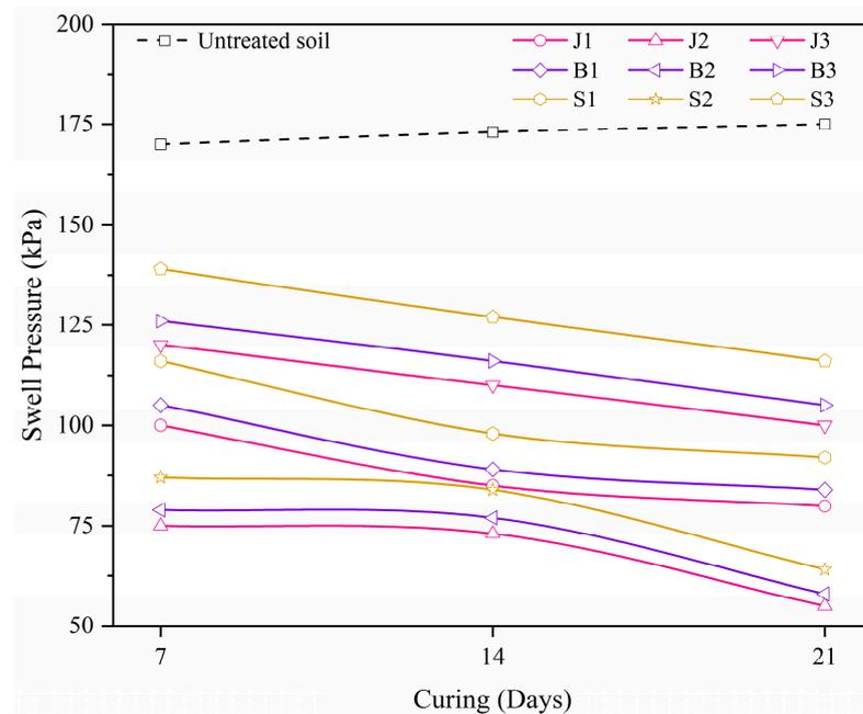
**Figure 14.** Swell test results of black cotton soil treated with enzyme solutions.
