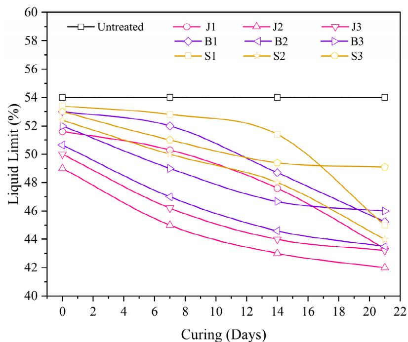
Figure 4. Liquid limit variation of soil 2 treated with enzyme solutions.
