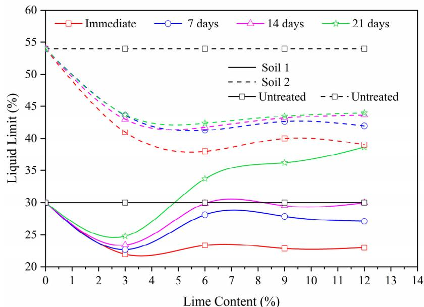
**Figure 5.** Liquid limit variation with lime content at different curing periods for soil 1 and soil 2.
