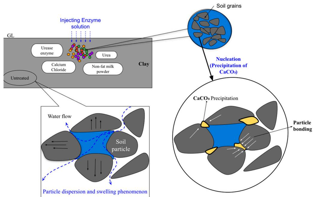
**Figure 10.** Schematic representation of EICP phenomenon in the soil pores.
