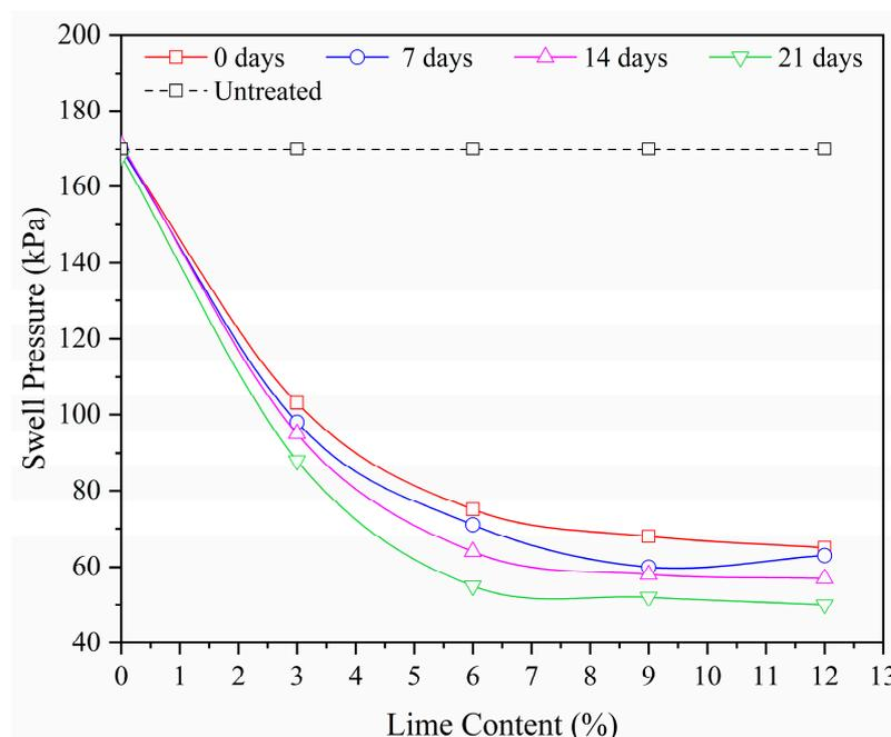
**Figure 16.** Effect of lime dosage on the swell pressure of black soil.
