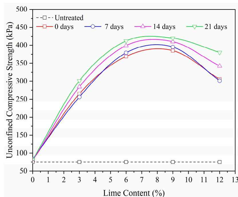
Figure 11. Strength variation in lime-treated red soil at different curing periods.
