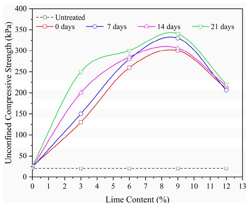
**Figure 12.** Strength variation in lime-treated black soil at different curing periods.
