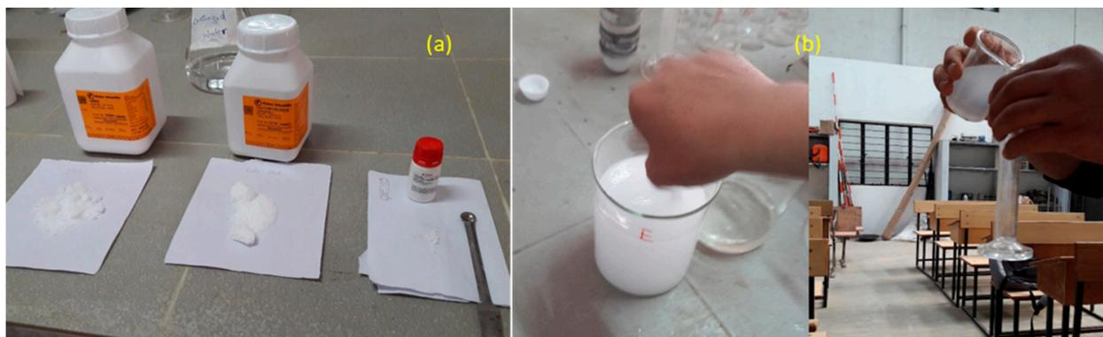
**Figure 2.** (a) Urea, calcium chloride, and urease enzyme. (b) Urease solution preparation.
