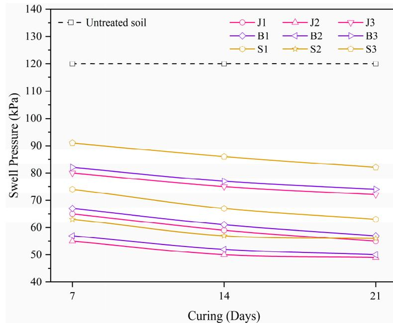
**Figure 13.** Swell test results of red soil treated with enzyme solutions.
