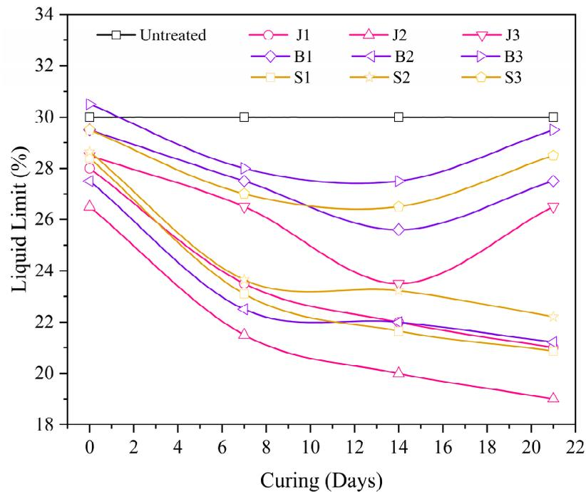
Figure 3. Liquid limit variation of soil 1 treated with enzyme solutions.
