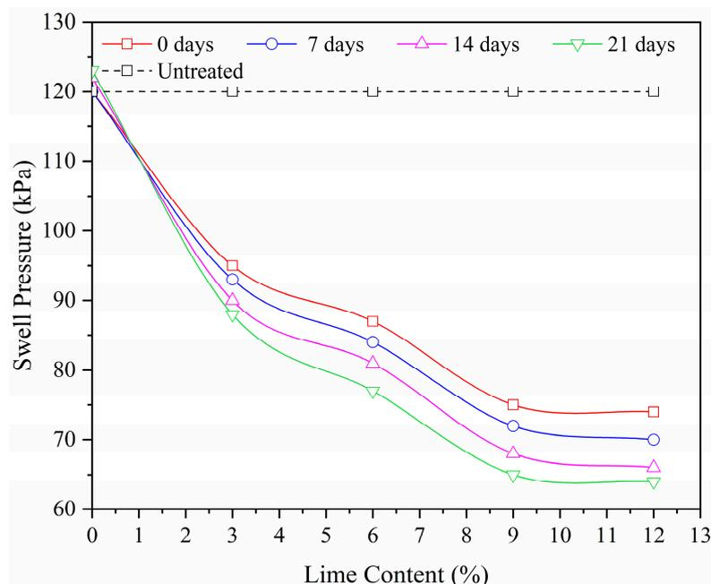
**Figure 15.** Effect of lime dosage on the swell pressure of red soil.
