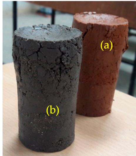
**Figure 8.** Failure patterns observed in the UCS tested: (a) red soil and (b) black cotton soil.
