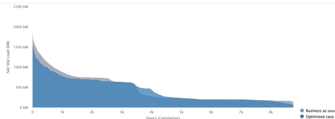
**Figure 25.** Peak load reduction occurs when the technologies recommended by the REopt web tool are implemented at Beacon High School. Source: Own elaboration.
