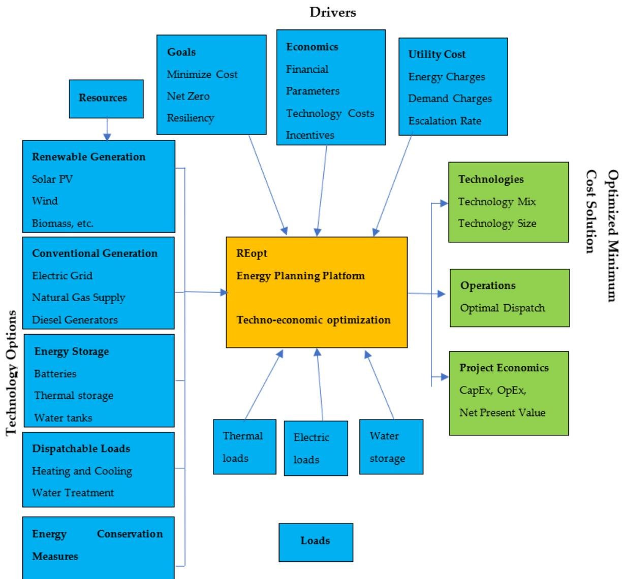
**Figure 1.** Steps of the general research methodology in a summary of the main inputs and outputs of the REopt model. Source: Adapted from [2].
