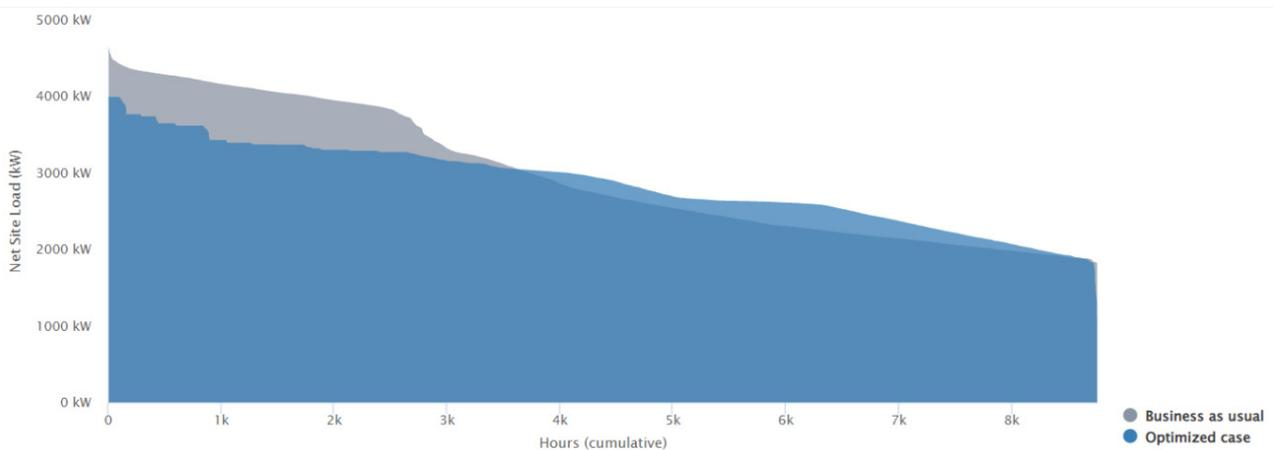
**Figure 19.** Reduction in peak load using REopt web tool optimization and the technologies recommended for Palomer Medical Center Escondido. Source: Own elaboration.
