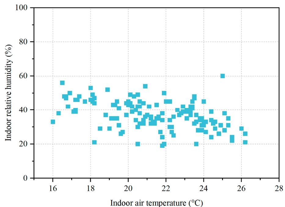
Figure 4. Environmental parameters: indoor temperature and relative humidity.
