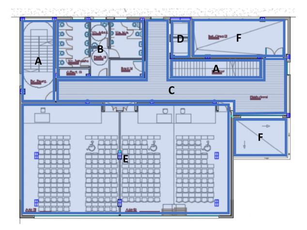
Figure 6. Example functional spaces ((A). Staircase, (B). Lavatory, (C). Corridor, (D). Lift, (E). Classroom, (F). Terrace).
