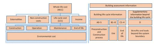
**Figure 1.** Categories of overall life cycle cost: on the left-hand side according to ISO 15686-5, and, on the right-hand side, EN-15643. In the blue box, the life cycle cost.
