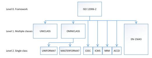
**Figure 2.** Hierarchical Structure of Classification Models. Abbreviations: Uniclass (UNC), Omniclass (OMC), Conseil Européen des Economistes de la Construction (CEEC), International Cost Management Standard (ICMS), New Rules of Measurement (NRM), and Andalusian Construction Cost Database (ACCD).
