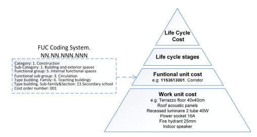
Figure 4. Cost structure, the work unit cost is obtained from the ACCD which is part of the functional cost.
